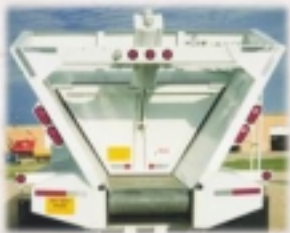
Concrete Modification Kit, (optional) for handling low-slump concrete. Includes a heavy-duty endgate with air-powered cylinder.
