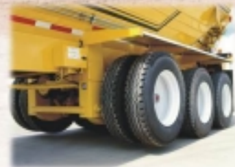
Air-Ride Suspension, (optional) also available with air-lift axes. Three-leaf suspension is standard.
